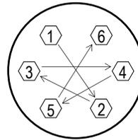
Tightening torque for center rod and out chambers.
